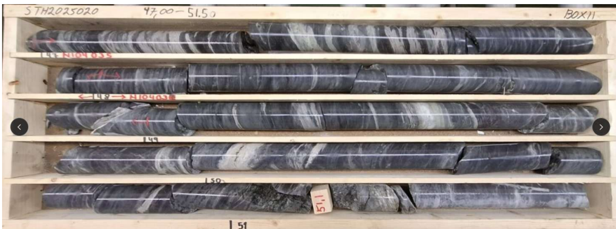
Figure 14: Photograph of drill core in drill hole STH2025020 displaying an excellent level of core recovery that is generally representative of all core drilled from the Stortjärnhobben deposit. Red annotations are used to mark the sample IDs and and black annotations for the meter marking intervals.
